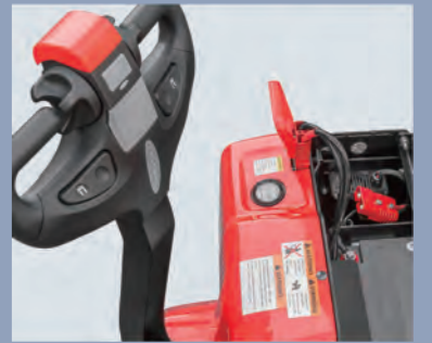
Features an optional built-in 50Ah charger and 150Ah AGM battery.
